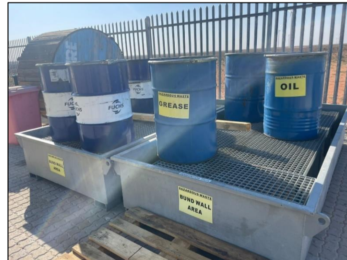
12. Used oils and grease temporarily stored with secondary containment to collect any spills / leaks
